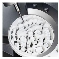
The R5 swivels the spindle (B axis) by up to  $\pm 35^{\circ}$ . This means that the workpiece holder only needs one moving axis (A axis) and gives the entire system stability.
